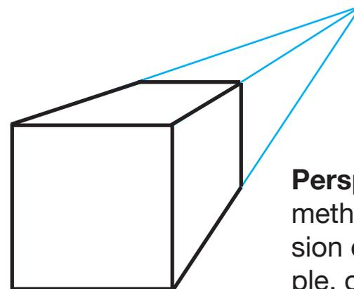
**Perspective:** A drawing method that create the illusion of space. In the example, one point perspective.
